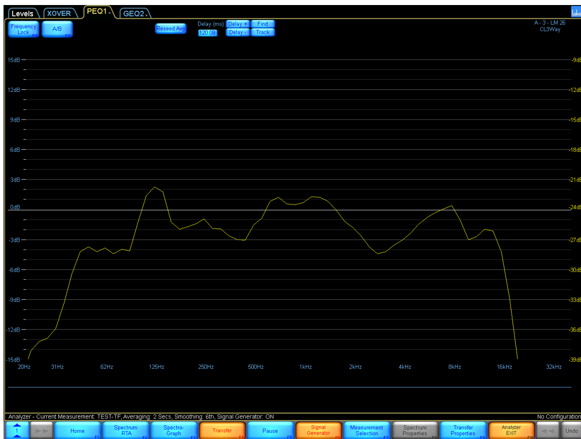
Figure 18-12: Transfer function measurement mode
