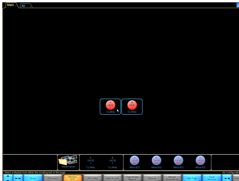
Figure 4-10: LM 26 Frame Placed in Main Work area
