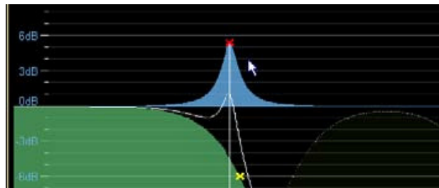
Figure 4-48: Adding a parametric EQ to the low channel
