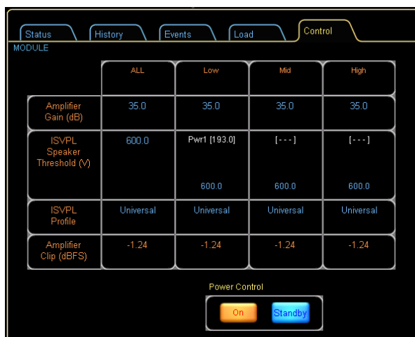
Figure 20-10: Control Tab with Parameters and Power Control
