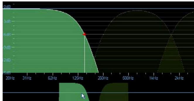
Figure 4-47: Splitting and moving the low channel HPF
